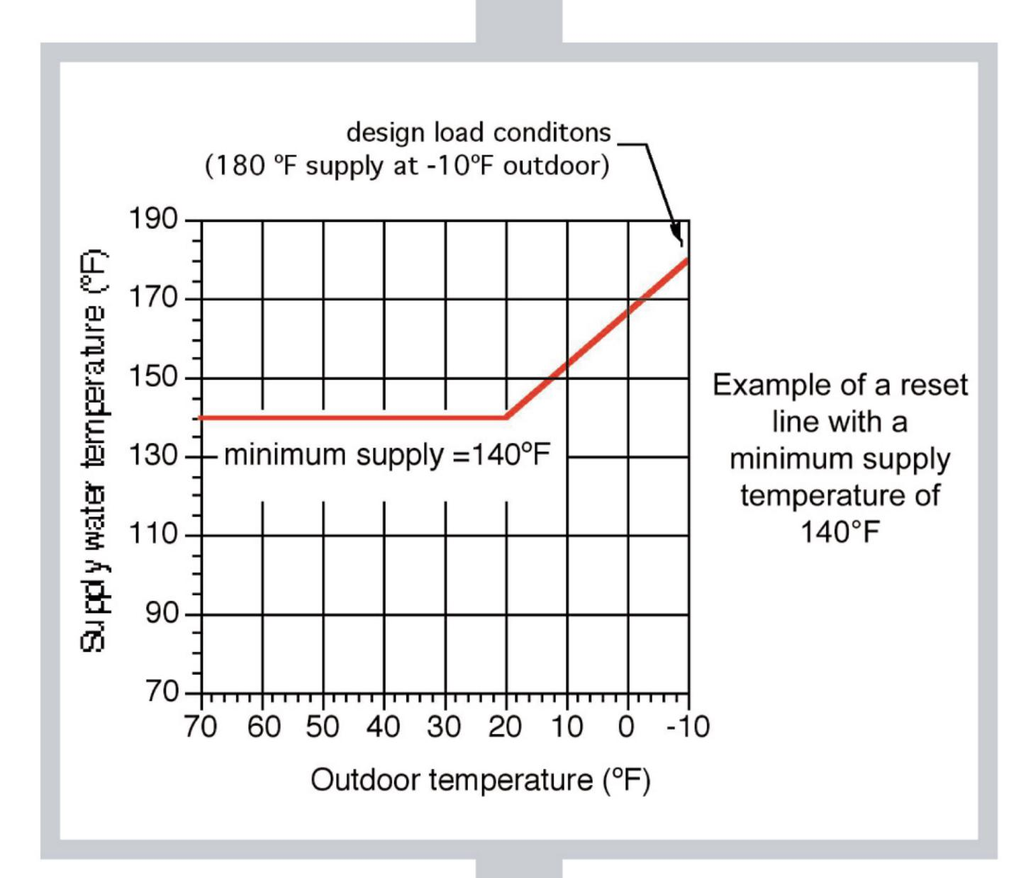
**Notice** how the lower portion of the sloping line has been "truncated" by the minimum supply temperature setting.
