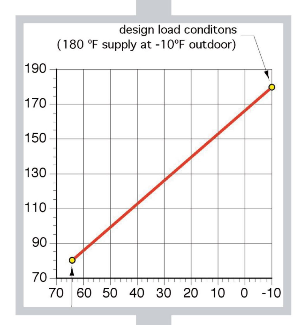
the energy savings mentioned as one of the benefits of outdoor reset control. These saving are mostly the result of lower heat losses from the boiler. If boiler reset is used as the sole means of water temperature control to the panel radiators it also improves comfort, especially during partial load conditions.
